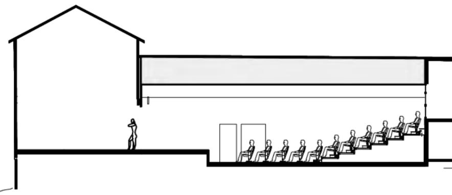
RETRACTABLE - RAIL MOUNTED - 260 high steps 900 deep deck x 6
